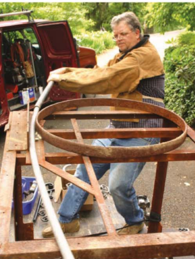
Greg Fagg and his homemade, wagon wheel bar bender.
